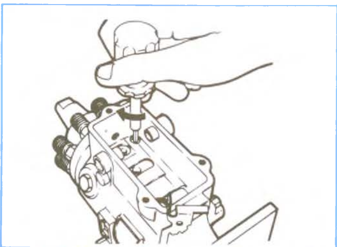
Figure 4-136, Installing Vent Wire Assembly.
